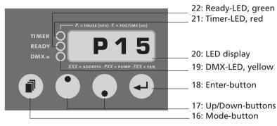
Abb. 1: Display shown at adjusting the pump output
